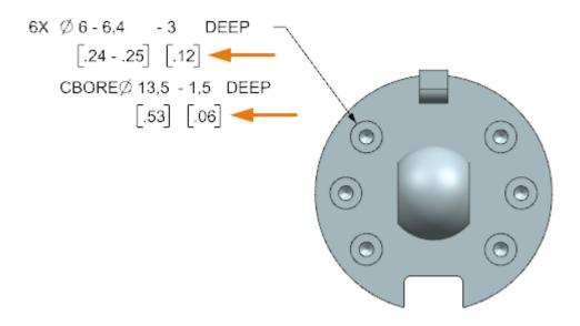
When you create or edit a hole dimension, you can set the Show Dual Dimension option for all supported parameters of the hole dimension. Prefix (diameter symbol) and suffix (depth text) for a hole diameter are displayed only for the primary parameters of the dimension.
