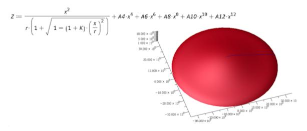
The new NX form element is connected to the corresponding Symbolica output worksheet and the STL output file of the 3D plot. Each time the Symbolica worksheet is changed, the linked NX facet body is updated.
