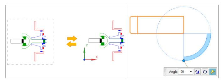
Once you have created a spline path, you can use the new Assign Tangency and Remove Tangency context menu commands to assign or remove tangency at any spline point. The spline path is automatically updated to reflect the tangent condition you selected.
