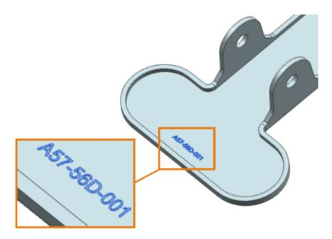
The resulting Print Mark text form element can be aligned and has an attribute that identifies it as special dynamic text. You can use asterisks (\*) as placeholders for variable text, which is replaced by single characters or digits in the string during additive manufacturing.
