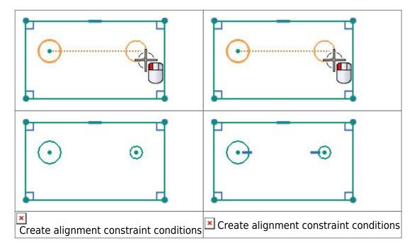
If Create Alignment Constraints is enabled, you can manually disable alignment constraints in the Inferred Dimensions and Constraints dialog box. If the user default is disabled, the Horizontal Alignment and Vertical Alignment options are not displayed in the dialog box.
