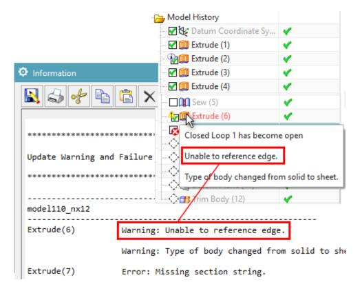
The default setting Warn on Missing References and the existing default setting Make Current Feature on Error together replace the function of the Edit During Update (EDU) dialog box that is no longer used.
