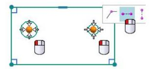
In this example, a second circle is placed to the right of the left circle. Note that the center of the second circle snaps so that it is aligned horizontally with the first circle. However, a horizontal constraint is only determined automatically if the user standard Create Alignment Constraints is set.
