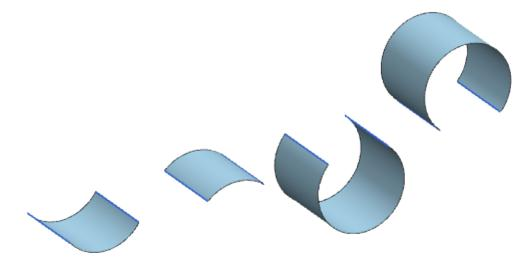
• Cubic type with Fillet Bridge mode - NX adds poles only when needed to achieve the desired consistency. In addition, handles are added to the defining edges of the surface so you can adjust the surface interactively. In the example below, the surface on the left has consistency G1 (G1) on both sides. The surface on the right side shows the pole structure when you change the consistency of the right side to G2 (G2).
