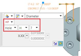
When you apply a boundary and fitting tolerance to a hole callout, the entire dimension above or inside it is displayed with the dimension line. You cannot apply the Split by Dimension Line setting to the dimension to display it both above and below the dimension line. When will this function be used?
